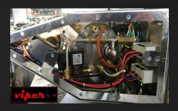
Our group is dry. When extraction is commanded, in a few tenths of a second the water is "called" from the boiler to the heat exchanger and corrected in the desired temperature in a few tenths of seconds before extraction. This guarantees an unsurpassed thermal stability.
