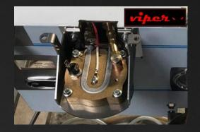
The final temperature is refined in the exchanger which overhangs and heats the group.
